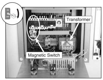
**Figure 53.** Magnetic switch inside the switch box.
